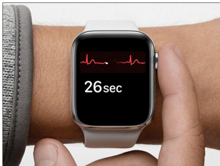
Figure 1: Image showing the Apple Watch ECG function in use. The participant has placed their right index finger on the Digital Crown to start the recording
