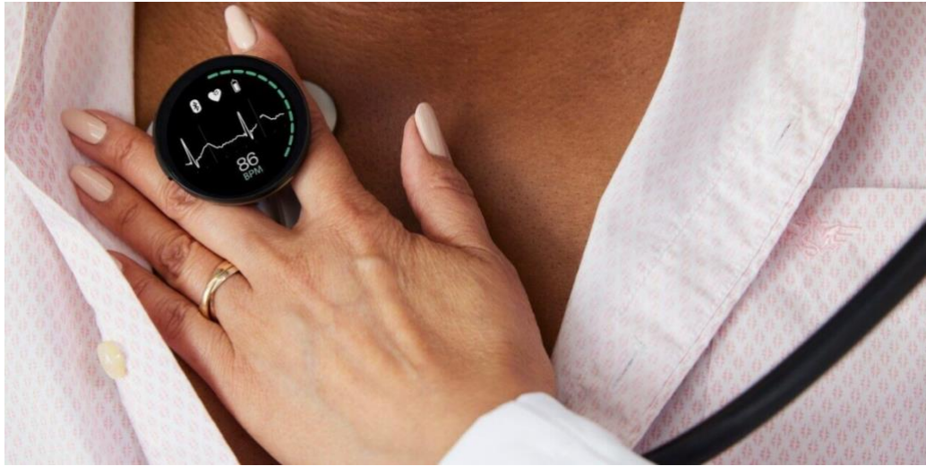
Figure 4: Image showing the Eko CORE 500™ digital stethoscope being used to record ECG data. The chest piece has been placed at the right upper aspect of the breastbone. For this study, the chest piece will be placed on the other side.
