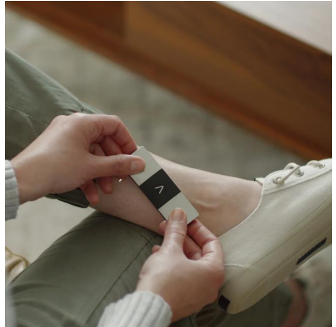
Figure 3: Image showing the KardiaMobile 6L device ECG function being used in 6-lead mode. Both thumbs are placed on the top electrodes. The bottom electrode is placed on the left ankle.
