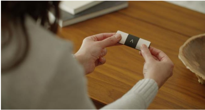
Figure 2: Image showing the KardiaMobile 6L device ECG function being used in single-lead mode. Both thumbs are placed on the top electrodes.
